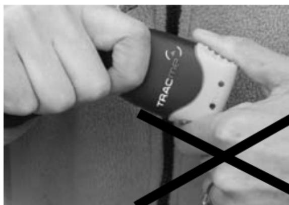
*The TracMe cannot be activated by holding onto the dark blue outer case.*
